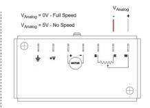
CAUTION: When using an analog command option, note that any improper connection may result in motor runaway or no motion control. Be sure not to exceed 5V input or damage to the control can result.
